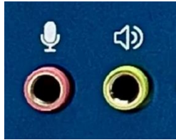
Audio connector: Microphone IN, Speaker OUT
