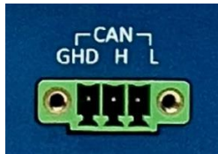
CAN Bus connector: GND, CANH, CANL
