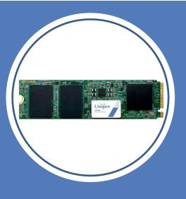
**Unigen Oncilla SSDs** offer blazing speed with next-level high endurance 3D eTLC NAND (480GB -3.84TB) and a PCIe® Gen4.0. NVMe<sup>™</sup> 1.4 controller that unlocks sequential read/write speeds of up to 7400/6700 MB/s in a space efficient design. With a 5-year warranty and up to 2400TBW Endurance for the 3.84TB design, these SSD's are built to last and offer plenty of space for your applications and data.
