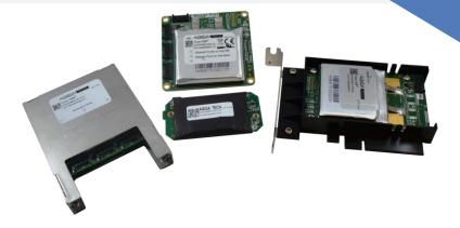
PowerGEM® is a Green Energy Module providing reliable back-up power for NVDIMM-N nonvolatile memory modules. Based on supercapacitor technology, PowerGEM modules offer a safer and more environmentally-friendly alternative to batteries. PowerGEMs also conduct real-time in-system health monitoring and tracking for a highly reliable solution that will operate over the system's life without conditioning or replacement.
