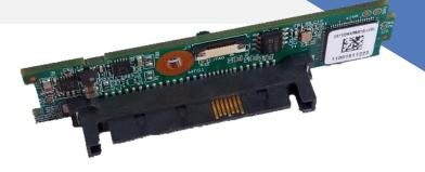
The Unigen SAS-to-SATA Interposer offers a cost-effective solution to enable high-capacity SATA drives to be used in enterprise storage systems that demand full-duplex active-active operation and redundant high-availability (HA) connectivity. This small form factor board provides two integrated SAS target ports and one integrated SATA host port, allowing standard single-port SATA HDDs or SSDs to function as dual-ported SAS SSP target devices.
