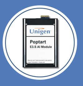
The Poptart E3.S uses two Hailo-8 Edge Al processors, featuring up to 26 tera-operations per second (TOPS) each. With an architecture that takes advantage of the core properties of neural networks, the Hailo-8 neural chips designed onto the E3.S allow edge devices to run deep learning applications at full scale more efficiently, effectively, and sustainably than other AI chips and solutions.
